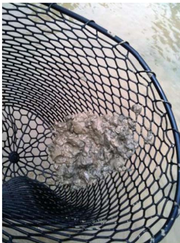
Figure 7. Net sample of bottom mud (typical) from four proposed dredge areas inside Hawai'i Kai Marina comprised primarily of silt.
